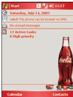
Fig. 11: VITO FindMe is a Today screen plug-in that provides an automatic reply with the device's location.
