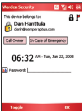
Fig. 2: The locked screen offers one-touch buttons to call the phone’s owner (you) or an emergency number.
